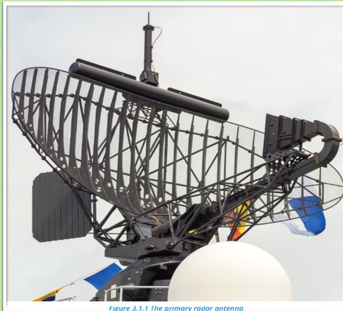
Figure 3.1.1 The primary radar antenna
