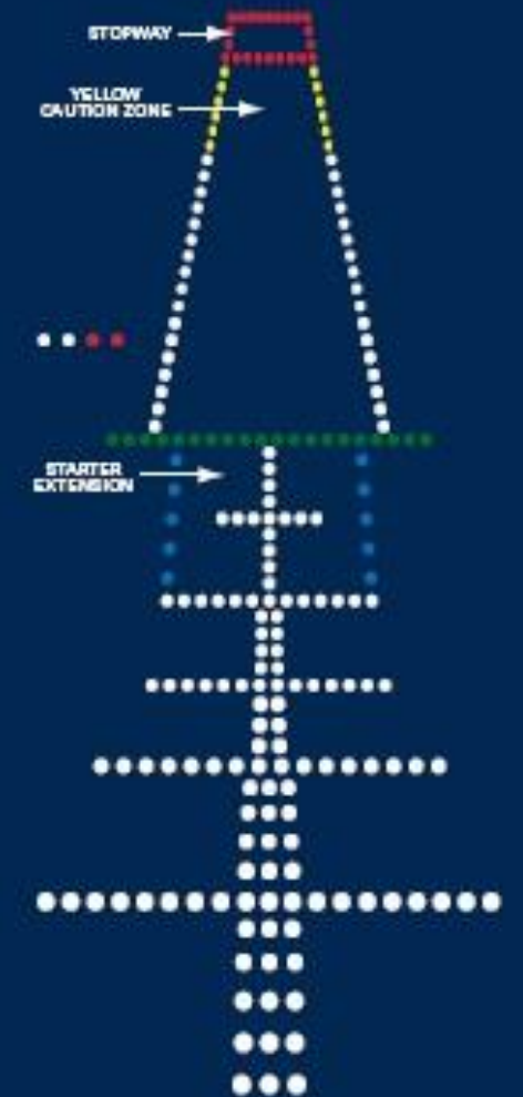
APPROACH AND RUNWAY LIGHTING TYPICAL CAT I SYSTEM SHOWING TAKE-OFF STARTER EXTENSION AND STOPWAY LIGHTING
