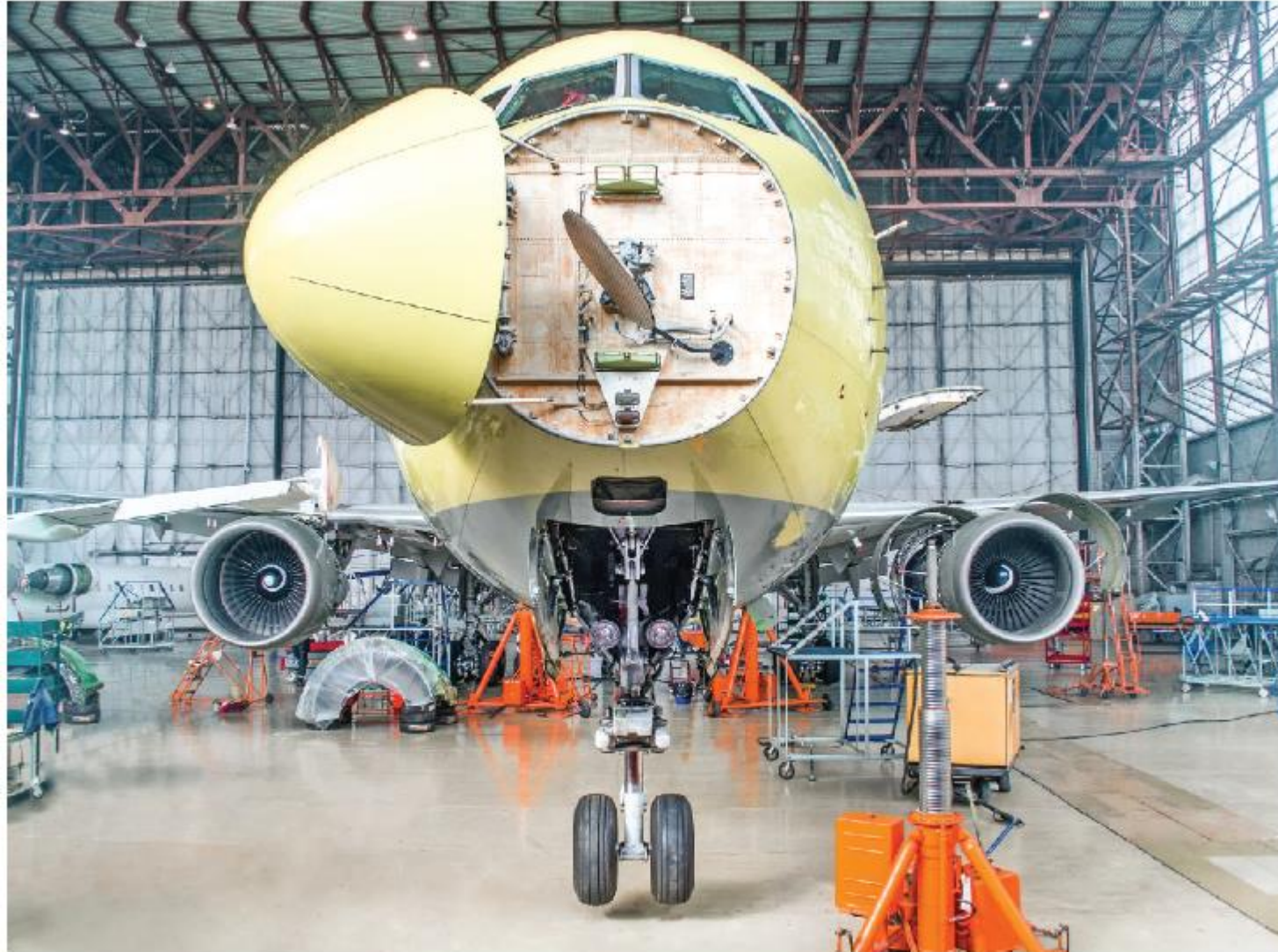
Figure 2.10 Example of firewall bulkhead
