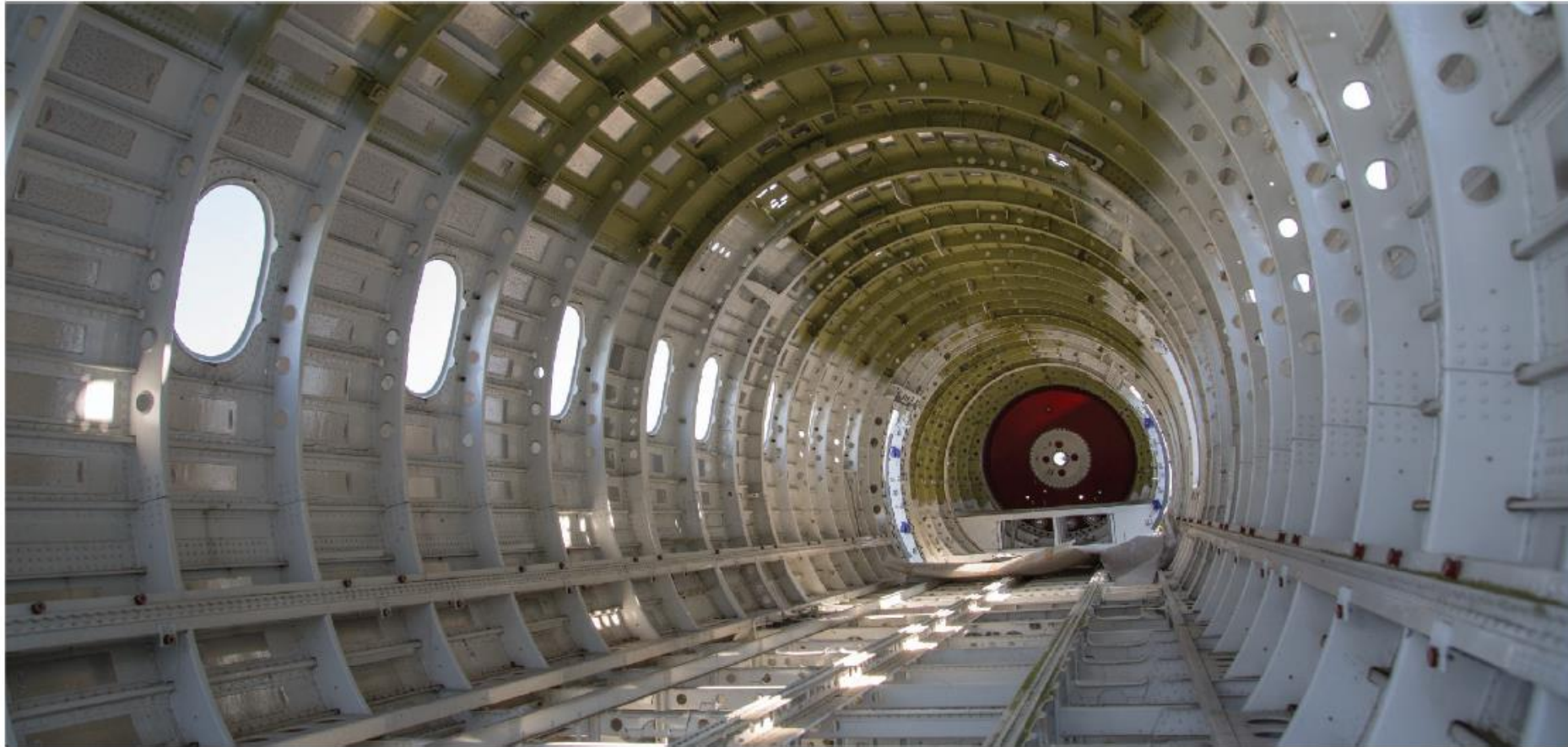
Figure 2.7 Semi monocoque fuselage
